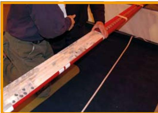
The wooden landing strip needs to be slightly narrower than the poles to ensure there is not an overhang (causing sharp edges on the sides of the bar).
