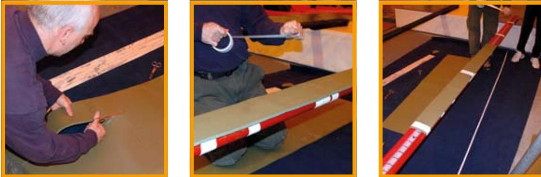
An alternative to a wooden landing area is to lay rope in the joins between the poles. This will fill the gaps between the poles. The rope only needs to be as long as you want the landing area to be. The rope is held in place with more silicon. It is optional to cover the landing platform with foam. It is more comfortable and safer for beginners or those working in bare feet but can be slightly less stable to land on
