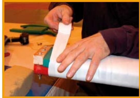
Taping is enough to hold all the rubber in place but extra glue can be used if you feel it is needed. The negative aspect of using glue is that, should a pole need to be replaced; the rubber will be destroyed when removed.
