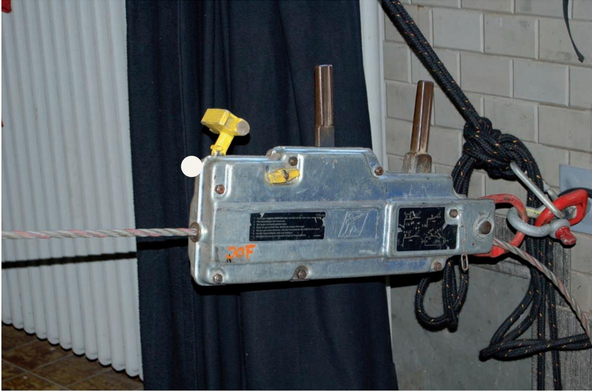
□ Tensioners (tirfor) can set the correct tension on the wire
